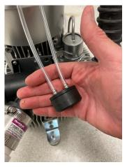
Hold Valve Firmly, Pull Off Tube
