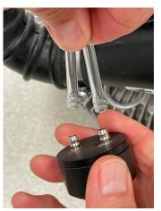
Hold Valve Firmly, and Push On Tube
