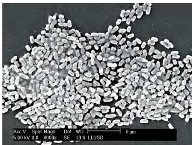
Fig. 2 Biofilm accumulated in control tubing: DI water and two-species inocula for four weeks.
