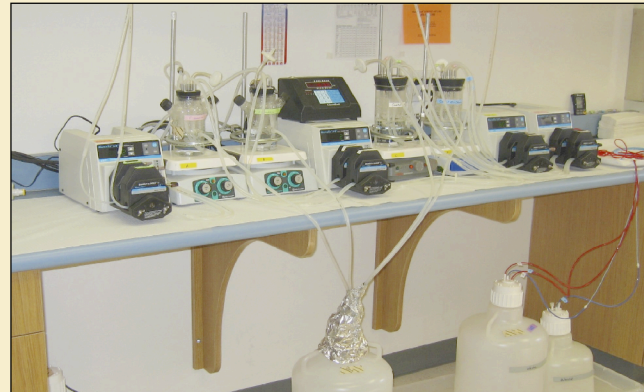
Figure 2. Dental Unit Water Line Biocide Test Model
