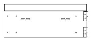
Back of System with Hinge Plates installed
