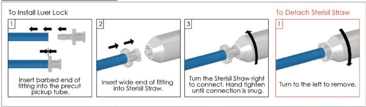
The Sterisil Straw comes with a Luer Lock. Proper installation of the luer lock is shown in the diagrams. It is important to cut the existing pickup tube to the proper length so that the bottom of the Sterisil Straw is at least a 1/4" from the bottom of the bottle.
