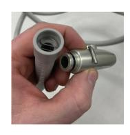
1. Remove the HVE tip, leaving the Clip and Coupler intact
