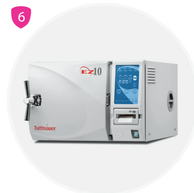
Steam autoclave for a minimum of 121 C (250 F) for at least 30 min, followed by a 30-min drying cycle.
