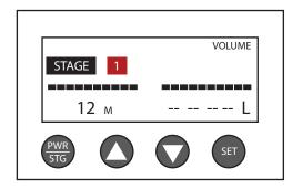
3. Once **Stage 1** is highlighted, press the SET button. The word 'set' should appear near the upper right corner of the screen. Note that the set mode will turn off if no buttons are pressed for 15 seconds. The SET button will then have to be pressed again.
