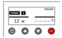
7. Press the PWR/STG button to get to Stage 2. Deactivate the months and liters timers. If the screen looks like the one on the left, skip to Step 16. If there are numbers for months and liters (for example, like the screen on the right), go to Step 8.
