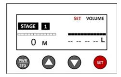
4. Ensure the black line is above month timer (left side). This line can be switched from side to side by pressing the PWR/STG button when the monitor is in set mode.
