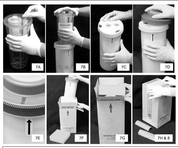
All packaging must be used to ship to recycler including all foam inserts in order to avoid leakage during shipment to the recycler facility.
