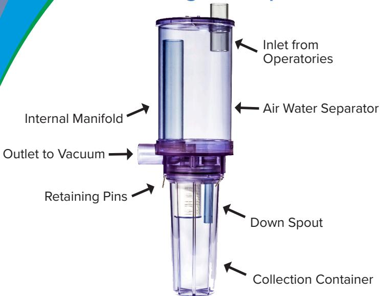
Your collection container must be changed once every twelve (12) months or when the sediment level reaches the full line on the collection container label; whichever occurs first. Check the sediment level of the collection container weekly.
