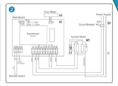
Follow-up time: The factory-made follow-up time of the suction system (dry vacuum system) is approx. 60 seconds. By turning the knob P2 on the timing relay, this running time can be adjusted.
