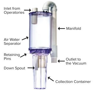
Your collection container must be changed once every twelve (12) months or when the sediment level reaches the full line; whichever occurs first. Check the sediment level of the collection container weekly.
